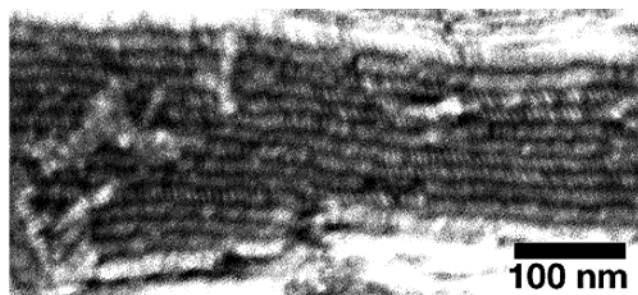
Figure 3. HRSEM image of \text{Cu}_2\text{S} nanorods self-assembled into a colloidal crystal.
